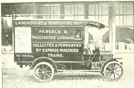
LANCASHIRE AND YORKSHIRE RAILWAY. Motor Van Corporation for the collection and delivery of parcels on the vicinity of Manchester. The cars have an 18 h.p. engine and can carry a load of 25 cwt.
